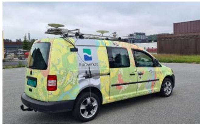
Figure 0-II: The Norwegian Mapping Authority vehicle with sensor platform
