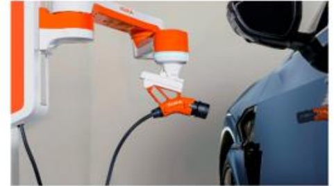
Figure 4-VII: Automated robotic arm charging an electric vehicle.
