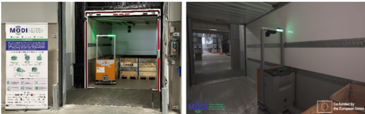
Figure 3: The Einride vehicle is being loaded by STILLs automated forklift. View from warehouse and from inside of the cargo hold.
