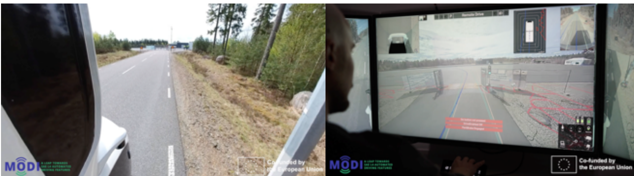
Figure 7: The Einride vehicle is approaching the closed gate (left). The gate has opened, the Remote Operator's view (right).
