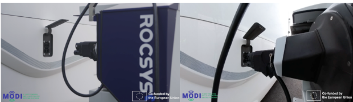
Figure 12: The Robotic arm moves a standard CCS charging connector (left) towards the Einride vehicle's charging inlet and connects (right).
