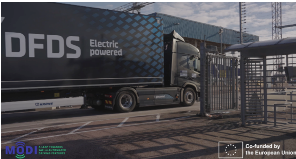
Figure 9: Upon the arrivals at Gothenburg RoRo Terminal, the truck performed a "digital handshake," automatically authenticating itself. The gate opened, and the specific container location was sent directly to the driver's app.
