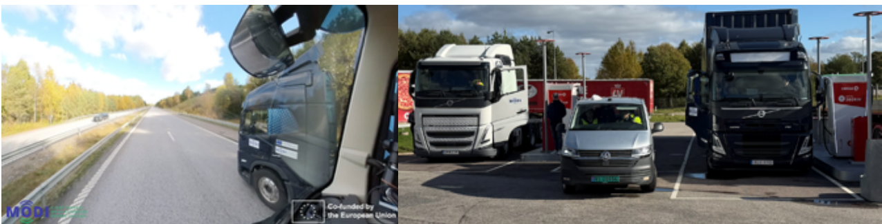
Figure 15: Successful demonstration of cooperative highway merging on the RV40 (left). The two Volvo trucks used for cooperative merging and passing, and the car from Q-Free used for "stationary vehicle" warning (right).
