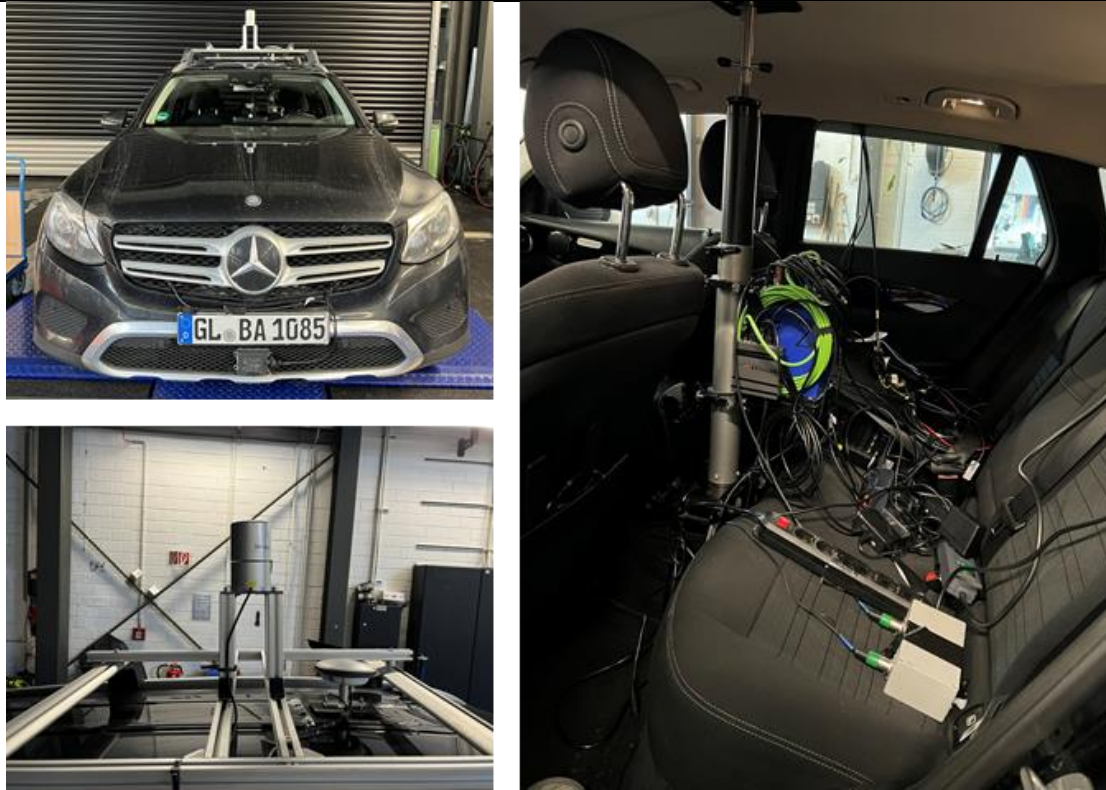
Figure 31: BAST passenger car equipped with LiDAR, Radar, IMU and dash cam
