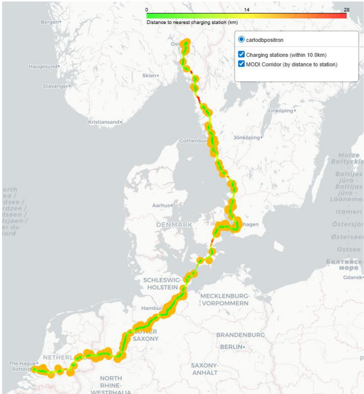
Figure 24: Charging stations and full MODI corridor, coloured by distance to nearest station
