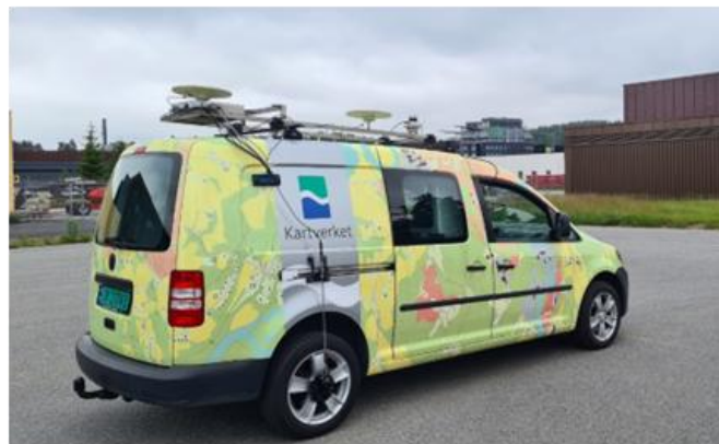
Figure 2: The Norwegian Mapping Authority vehicle with sensor platform
